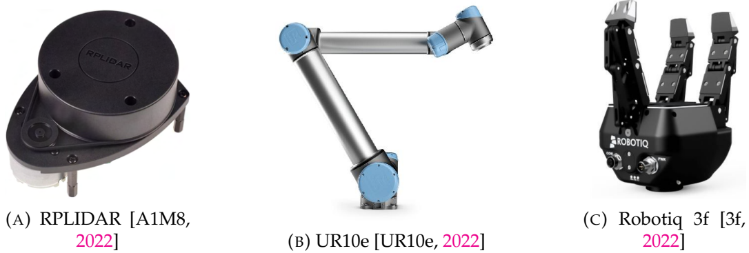
FIGURE 3.5: Laser scanner, arm and gripper in Amiga
